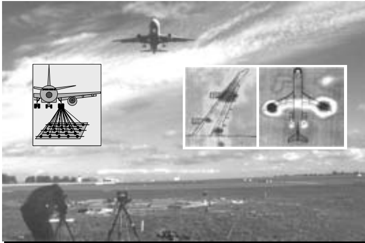
Fig. 9: Acoustic camera arrangement (inserts: schematic and noise maps)- Source DLR
