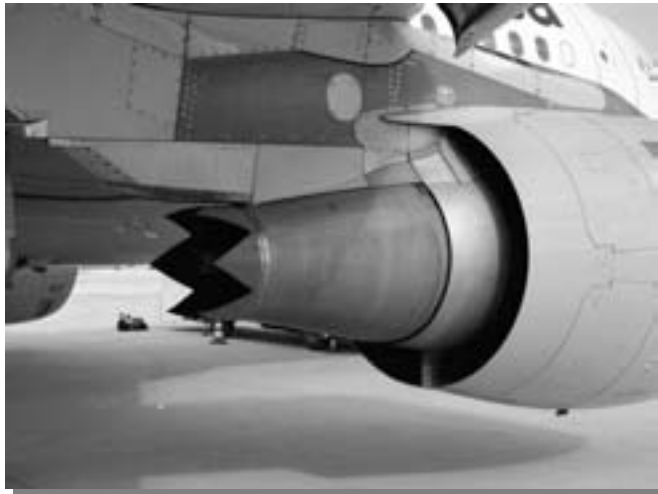
Fig. 7: A319 equipped with chevroned nozzle (DLR-Lufthansa project)
