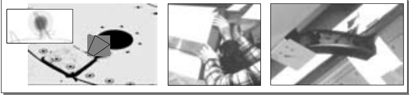
Fig. 11: Wing modifications to reduce noise of venting holes (left), edges (center) and track cut-outs (right) Source: DLR-Lufthansa
